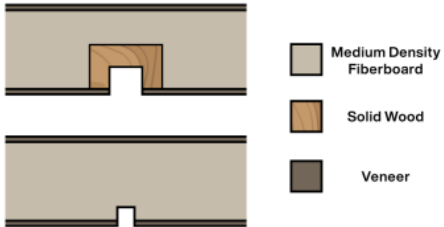
Figure 150 – Machining Through Veneered Panels
