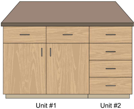
Figure 20 - Grain Layout, Flush Panel, Economy Grade
