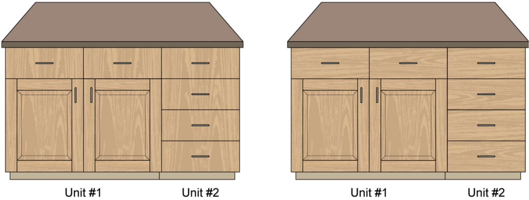
Figure 18 - Grain Layout, Stile and Rail 1
